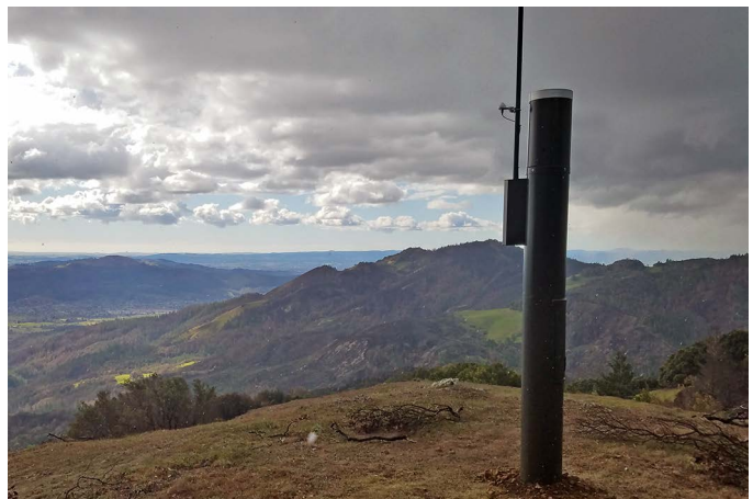
A new rain gauge upstream on Bald Mountain burn-scarred hillside
